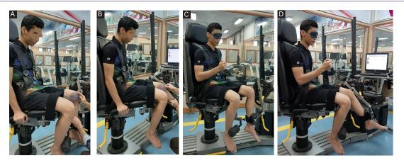
Figure 1. (A) Setting out the Starting Position (flexion 90). (B) Setting out the Target Angle Passively (Passive Positioning) With Eyes Open. (C) Starting Position of the Test With Eyes Closed. (D) Active Reproduction of the Target Angle With Eyes Closed.
