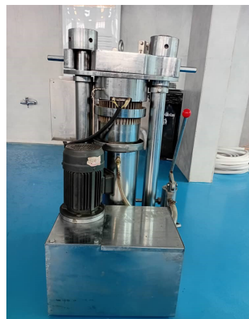
Figure 1. Laboratory-Scale Cold-Press Extraction System Used for Solvent-Free Recovery Of Chia Seed Oil.
